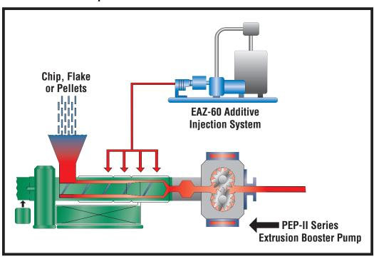
Zenith Pumps can handle all your extrusion pumping applications including additive injection for on-line compounding of tackifiers, colorants, stabilizers, etc.
