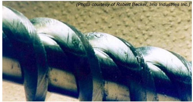
Figure 9 Pump Rotor Damage Caused By Hard Contaminant
