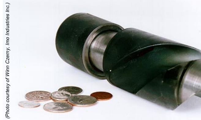
Figure 10 Running Clearance Increase Caused By Very Fine Contaminant
