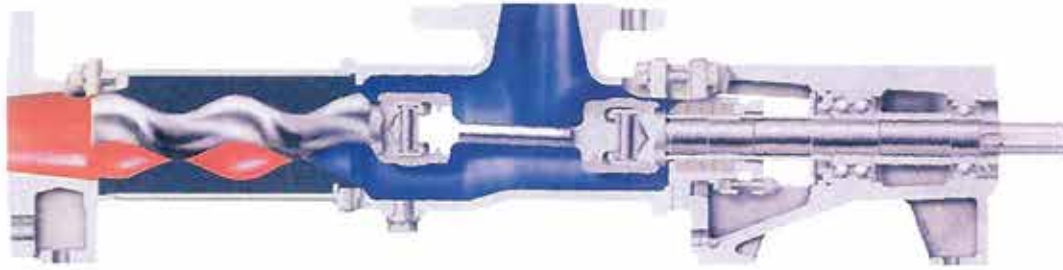
PROGRESSING CAVITY PUMP T1S
