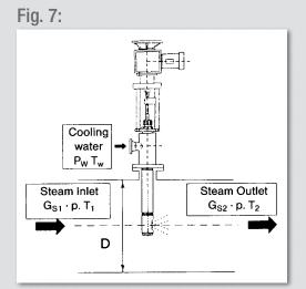
Calculation Calculation of the injection water quantity
