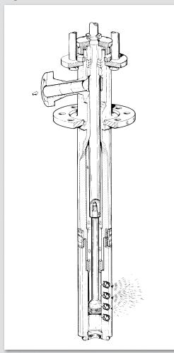
The nozzles in the sprayhead are designed to give the injection water a high velocity and a radial rotating movement under all conditions. The result is a fine atomisation and very quick evaporation. (See fig. 2)
