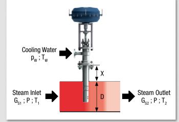
Fig. 7: D = diameter of steam piping
