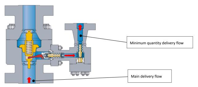
Figure 2 MRK valve with closed non-return plug and open bypasses
