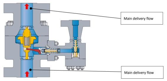
Figure 4 MRK valve with open non-return plug in maximum flow level and closed bypasses
