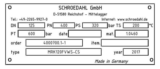
Figure 8 Example of a nameplate of the type MRK
