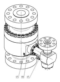
Figure 1 Sectional drawing and isometry of the valve type MRK (example)
