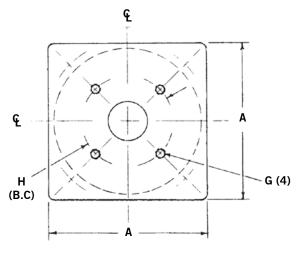
Blind mounting holes, drilled to accept furnished self-tapping screws Designed for use with  $\frac{1}{4}$ " thick solenoid mounting plate
