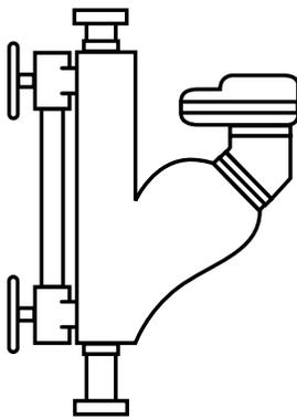
**It is extremely important that type of level control supplied and type listed in solid state controller be same.** Generator is factory shipped with matched types.
