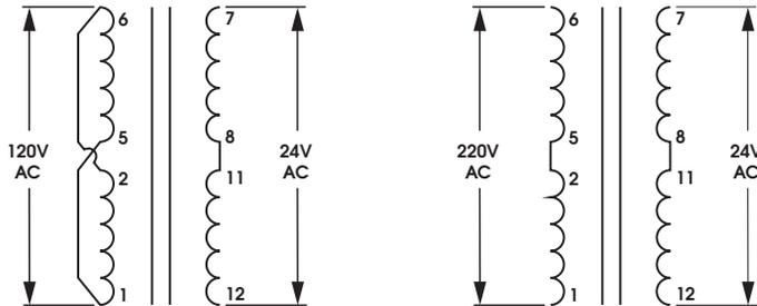
Panel is normally factory shipped for 120 Volt/ 1 phase/60/50 Hz. If so desired 220/1/50 or 60 Hz power can be used. To convert to 220 volt input it is necessary to reconfigure 24 volt output transformer. Below is wiring diagram for 120 volt and 220 volt input.
