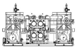
Self-priming, double entry, horizontal pump types
