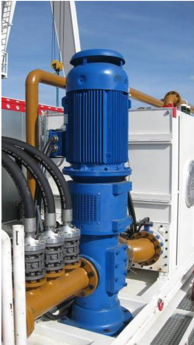
Allweiler screw pump of the “SN” series, used as filter oil and cooling system pump.
