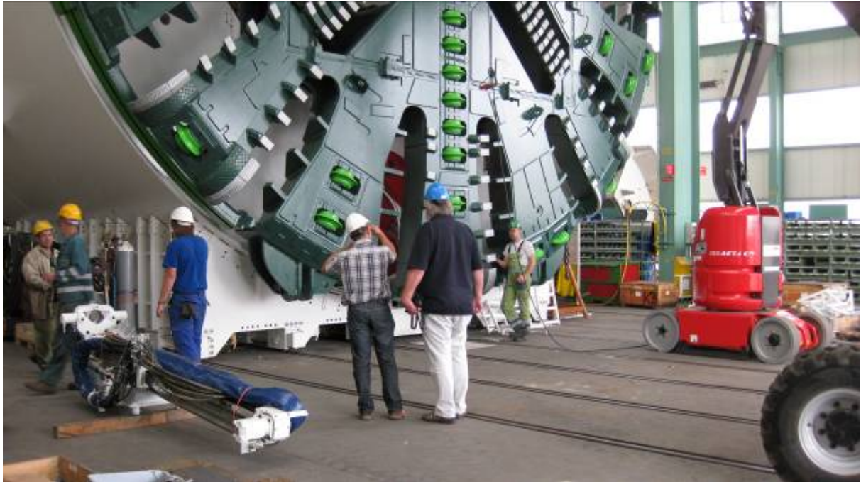
The lower half of the drilling head on a Herrenknecht machine under construction.
