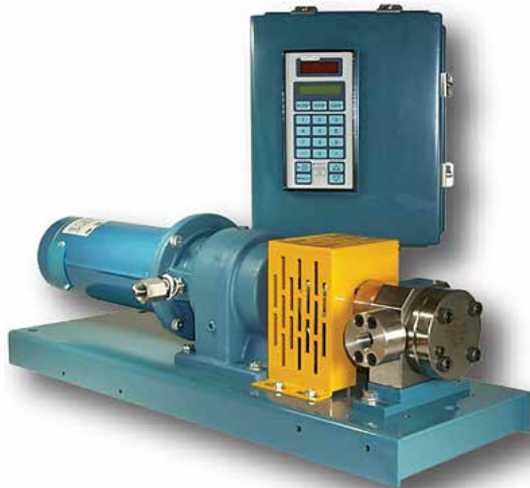
Image 2. Metered flow can be adjusted by simple speed control.
