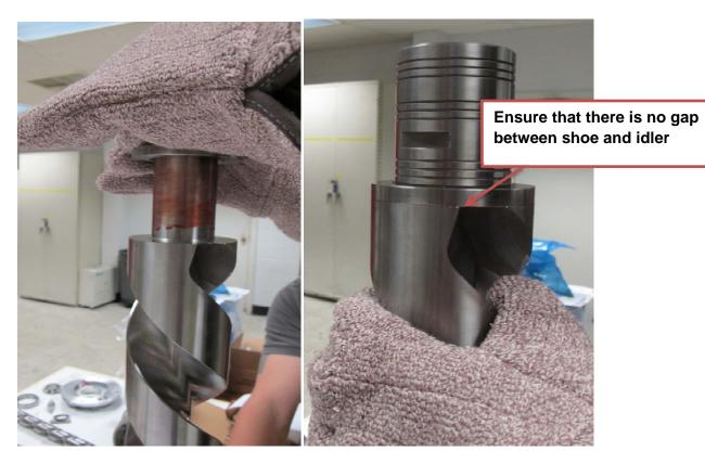
Slip the shoe onto the idler. Use arbor press to seat sleeve if necessary.
