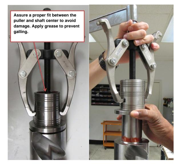
Use a gear puller to remove the shoe.
