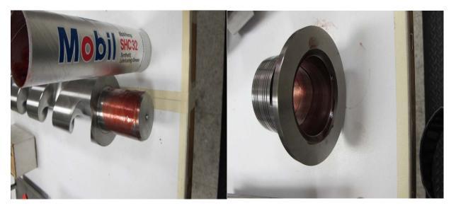
Clean mating OD of the idler rotor and apply high temperature grease, such as Mobiltemp SHC 32 grade.
