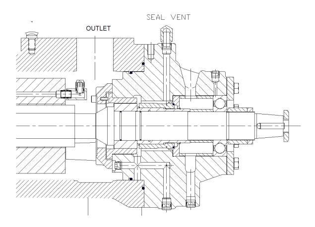
Filling or Venting Seal Cavity Using Seal Vent
