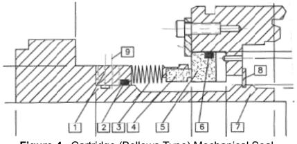
Figure 4. Cartridge (Bellows Type) Mechanical Seal
