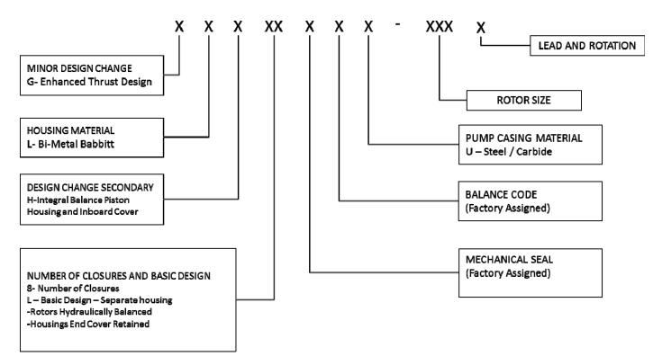
Figure 1. Definitions of Model Designators of GLH8L-630 pumps
