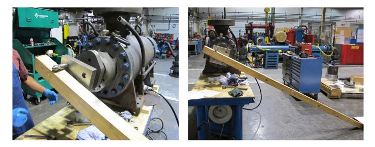
Above photos show proper way to lock shaft in position to break lock-nut free on shaft.
