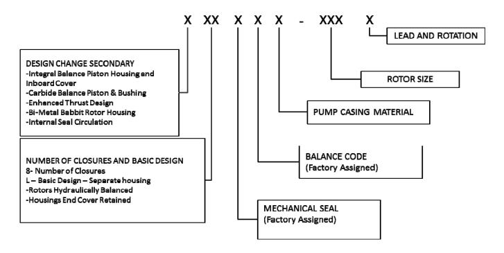
Figure 2. Definitions of Model Designators of J8L-630 pumps
