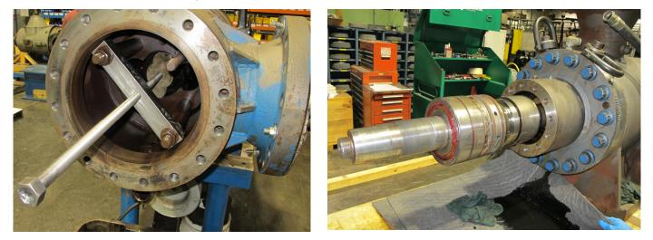
**LEFT** – Pressing power rotor out of inboard cover. If shaft is to be reused, ensure a blank is placed between power rotor removal strongback (S626MN) and outboard end of power rotor. **RIGHT** – Mechanical seal/bearing installation.
