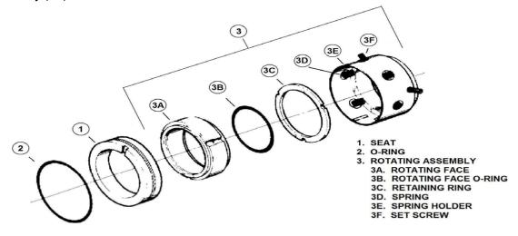
Figure 3. Mechanical Seal Drawing
