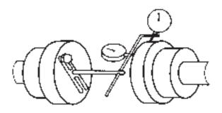
Figure 5.3: Alignment of the coupling with dial gauges
