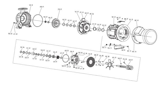
Design U3.3A-K1 (unbalanced mechanical seal with carbon-bearing)
