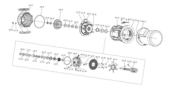
1A Design U2.1-S1 (balanced mechanical seal with SIC-bearing)
