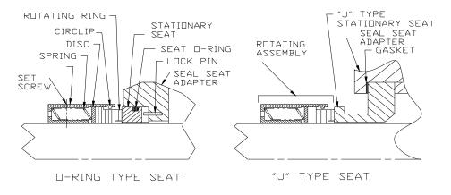
METAL BELLOWS MECHANICAL SEAL
