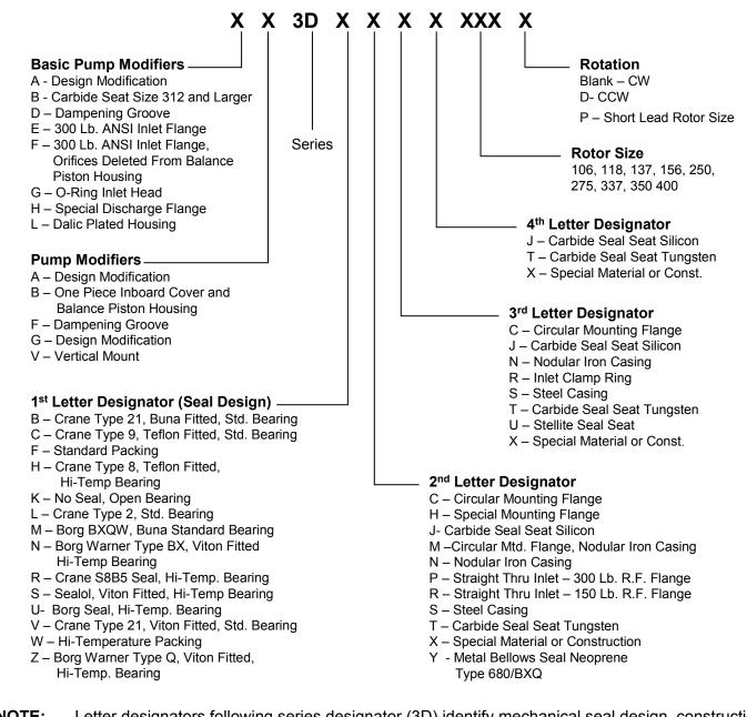
**NOTE:** Letter designators following series designator (3D) identify mechanical seal design, construction and special features. Series designator (3D) is followed by 1, 2, 3 or 4 letter designators. Examples of determining a particular pump type from letter designators are given below. Table applies to all designators.
