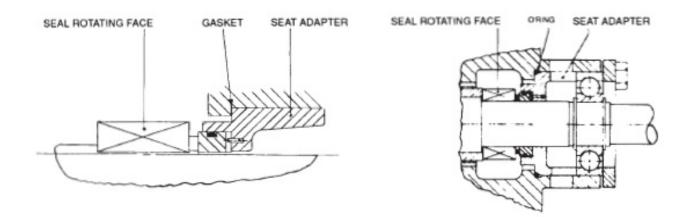
Figure 10. Seal Installation Variations
