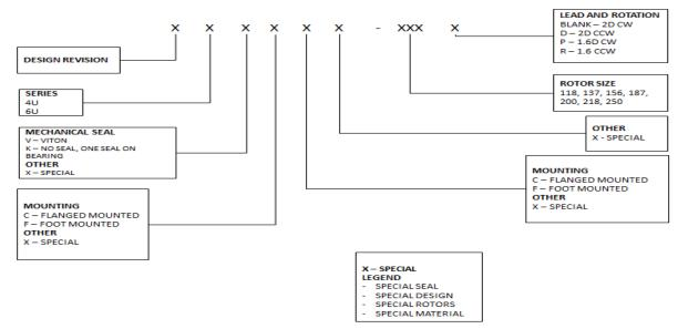
FIGURE 1. DEFINITIONS OF MODEL DESIGNATORS FOR SERIES 4U AND 6U
