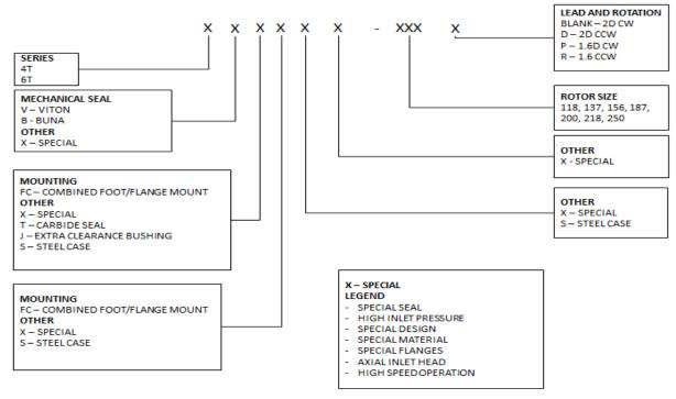
FIGURE 2. DEFINITIONS OF MODEL DESIGNATORS FOR SERIES 4T AND 6T
