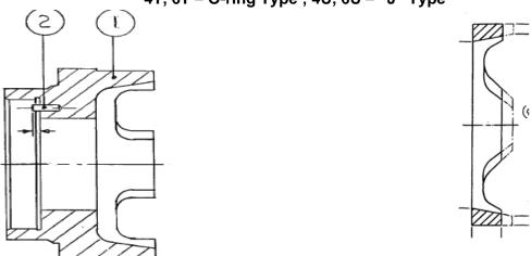
Figure 4. O-Ring Type Seal Seat Adapter
