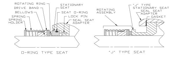
Figure 3. Mechanical Seal Drawing (Single Spring, Bellows Type)
