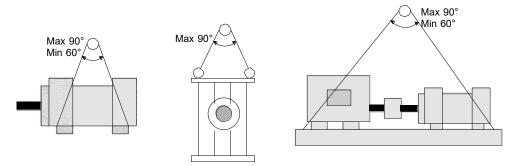
Figure 1 – Lifting Pumps and Pump/Driver Assemblies
