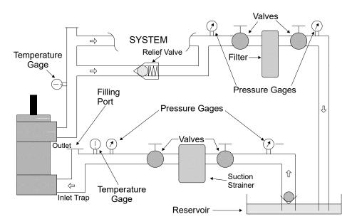
Figure 10a - Vertical Mounted Pump
