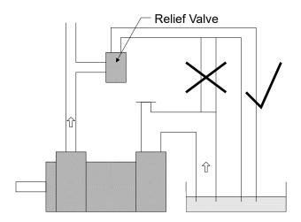
Figure 7- Proper Relief Valve Return Line Arrangement
