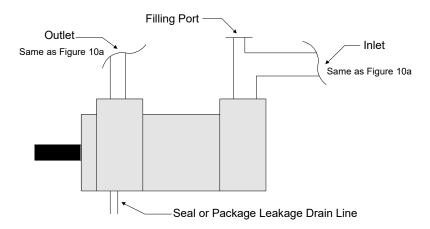
**Figure 10b - Horizontal Mounted Pump**
