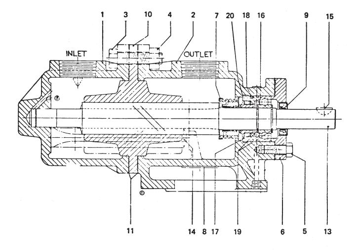
Fig. 1. Assembly of Series A313A Pump
