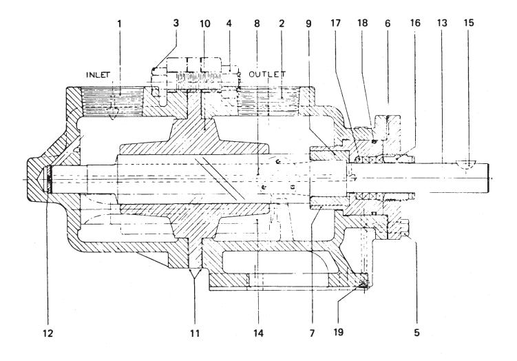
Fig. 2. Assembly of Series A313AD Pump
