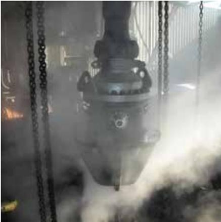
The innovative DeltaValve auto-switch coke cutting tool provides a high level of safety and reliability during de-coking operations by allowing the tool to remain in the drum during switching between boring/cutting modes. The auto-switch tool, in combination with the DeltaValve drill stem guide enclosure and the top unheading valve, provide maximum coker safety by allowing personnel to be removed from the cutting deck.
