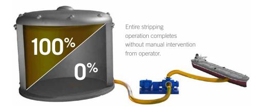
Once installed, its unique and patented technology measures cavitation directly from inside the pump in real time. Should any significant pressure reductions at the pump suction take place during unloading or stripping, the pump will continue to run at the fastest speed possible while still preventing cavitation or audible vibration.
