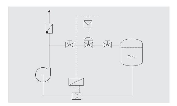
A flow sensor in the suction line, which senses the low flow conditions to the pump. Also available in a material as specified.
