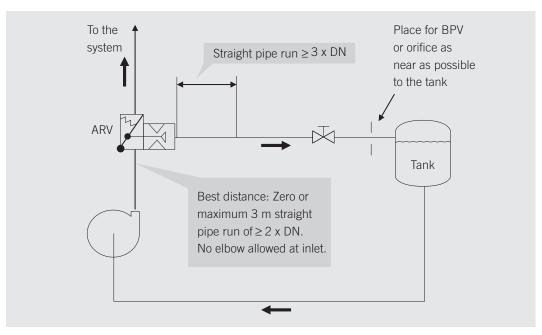
> **Note:** Vertical installaion of the ARV directly on the pump discharge is best!
