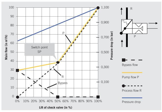
> Above flow curve shows the valve behaviour for the flow reduction process (shut-down event).
