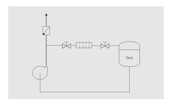
Also, a pressure reduction system has to be provided with orifice plates that are subject to cavitation and wear.
